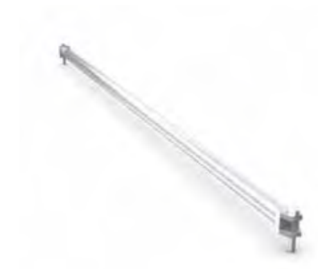
S4 BRACE 2000 mm (78,74") Aluminium tube ended with quick-locking jaws for horizontal bracing.
