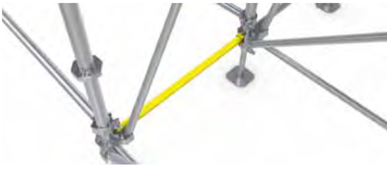
S4 BRACE 1000 mm (39,37") Aluminium tube ended with quick-locking jaws for horizontal bracing.
